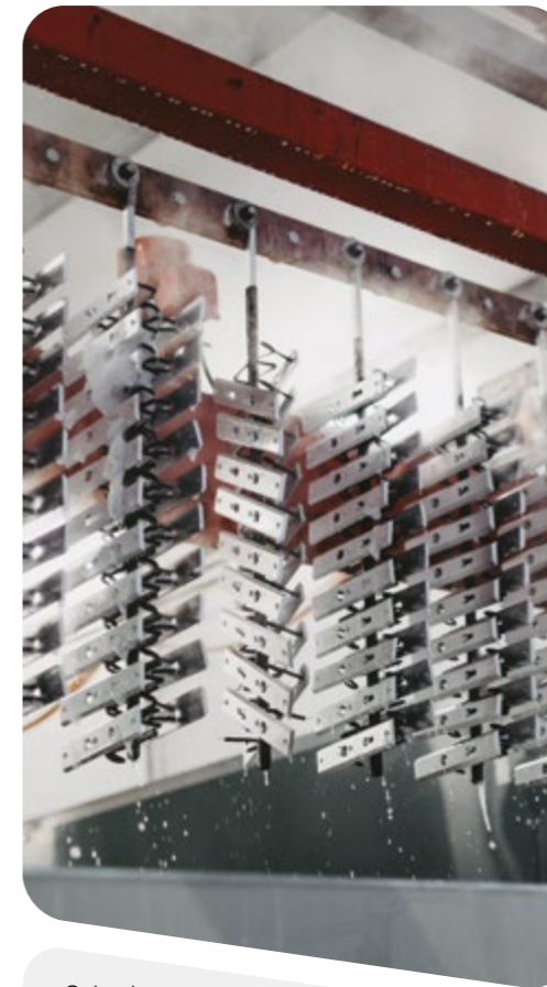
Colouring with the anodic oxidation method ensures longer product life; photo: AXA©.
